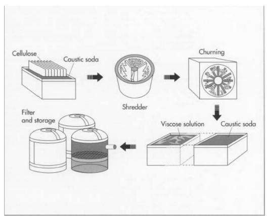
To make rayon, sheets of purified cellulose are steeped in caustic soda, dried, shredded into crumbs, and then aged in metal containers for 2 to 3 days. The temperature and humidity in the metal containers are carefully controlled.
